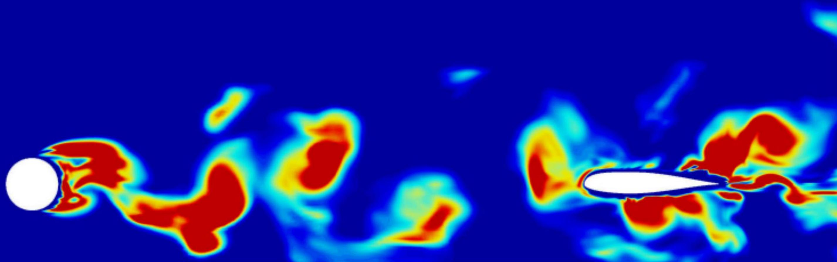
Virginia Tech leads the way in turbulence modeling and validation through combined computational/experimental research. Depicted: A benchmark flow case centered on unsteady transitional flows led to new eddy-resolving model implementation validated using high resolution, time resolved particle image velocimetry (PIV).
