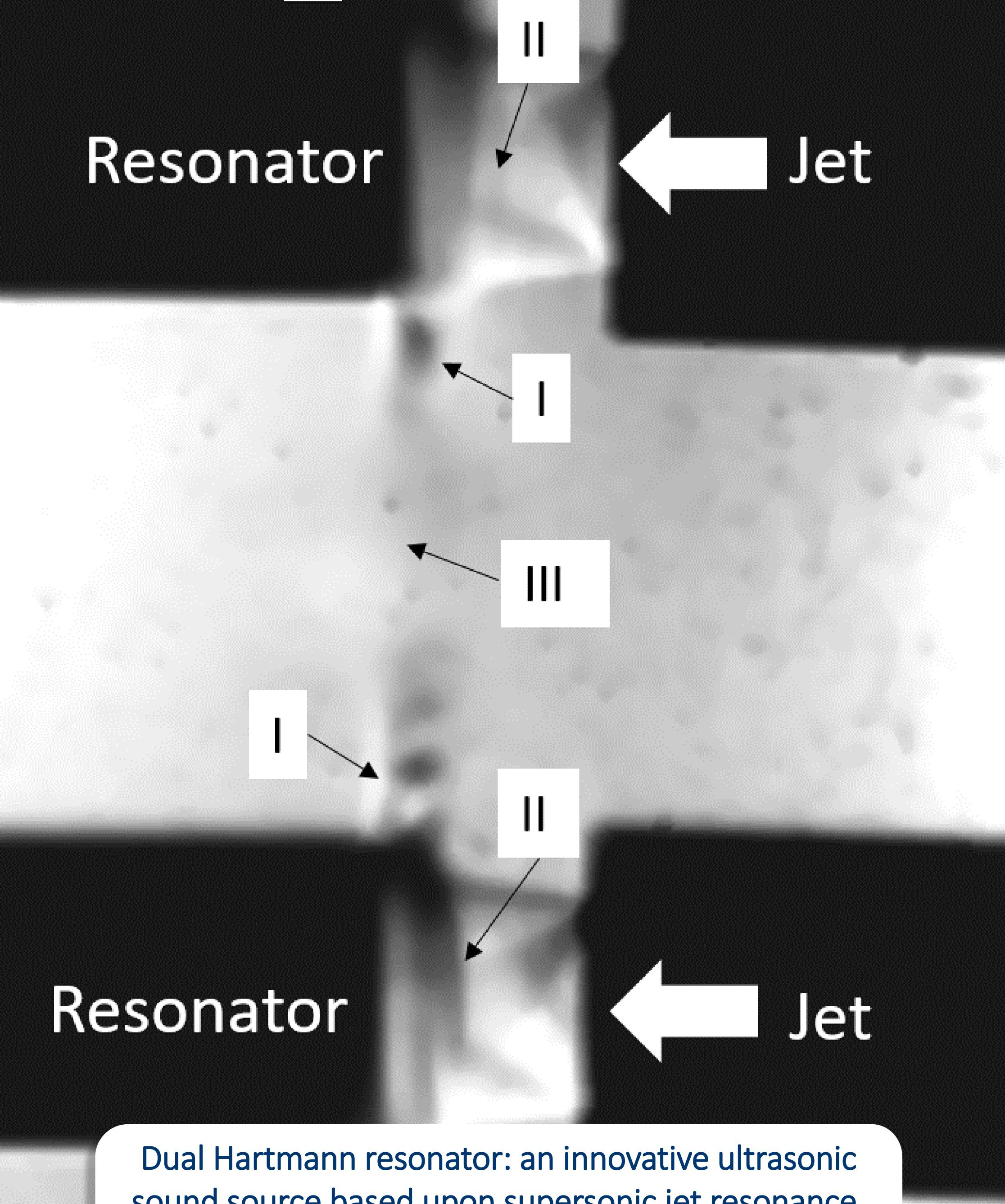
Dual Hartmann resonator: an innovative ultrasonic sound source based upon supersonic jet resonance. Produces 20 kHz sound at 120+ dB, enabling ultrasonic sensing of engine mass flow and thrust.
