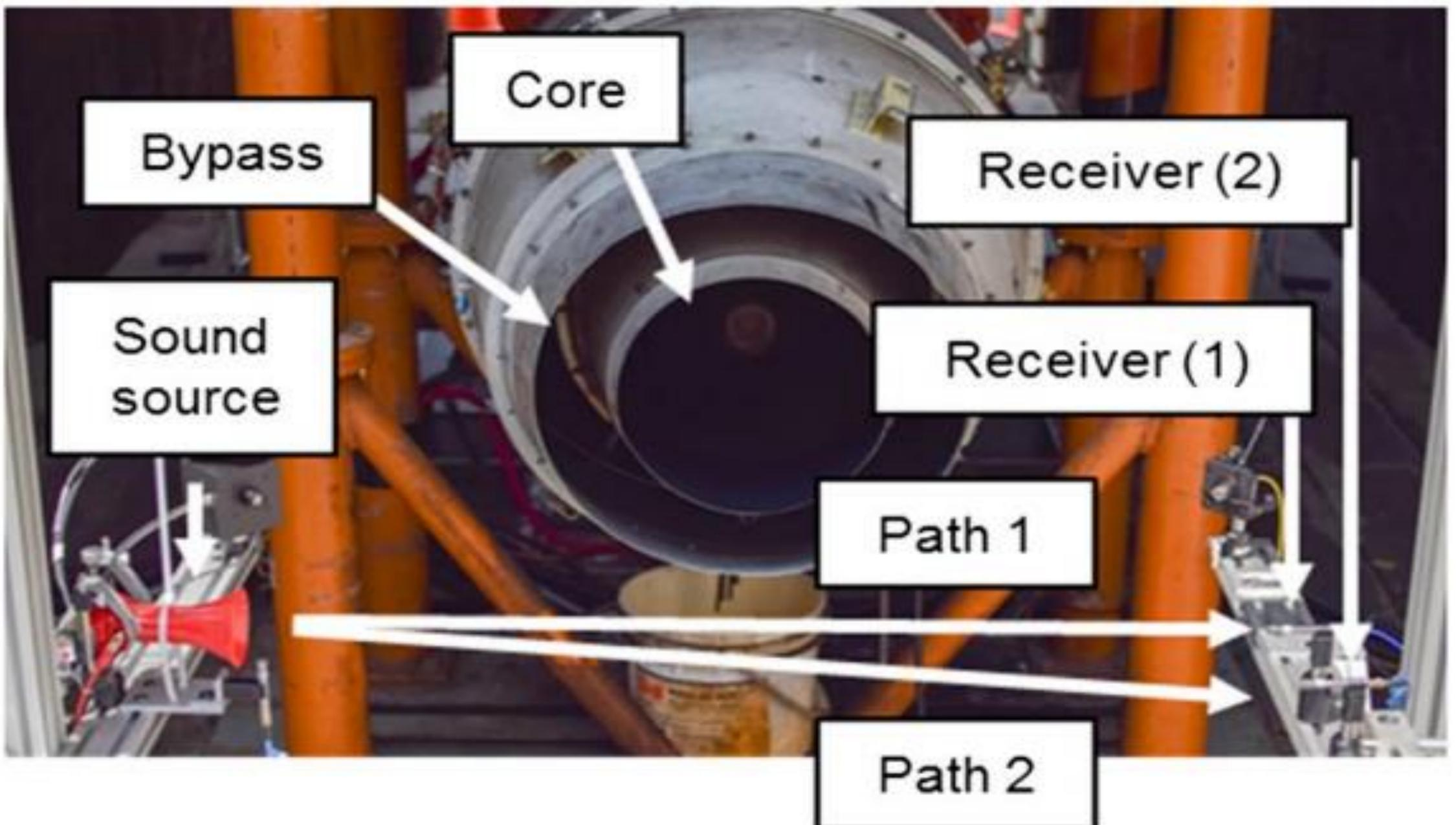
Virginia Tech, with the support of Rolls-Royce, has developed a non intrusive measurement technique to accurately determine engine thrust.
