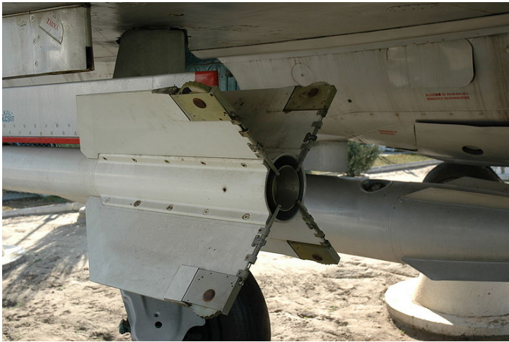
Figure 1. A photograph of the empennage of a high-speed missile (left) and a simplified illustration (right). Note the mechanical roll stabilization device embedded at the outer, trailing edge of each tail fin.
