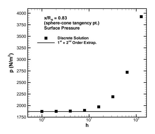
Fig. 6 Behavior of the surface pressure as the mesh is refined at the sphere-cone tangency point ( $x/R_N = 0.83$ ).
