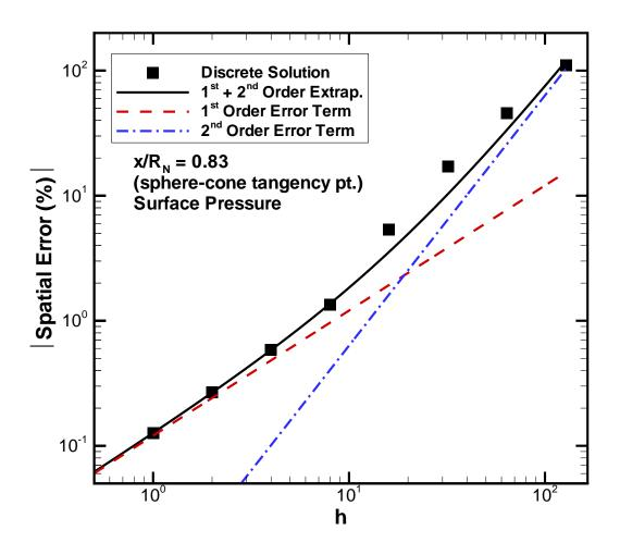
Fig. 7 Error in the surface pressure as the mesh is refined at the sphere-cone tangency point  $(x/R_N = 0.83)$ .
