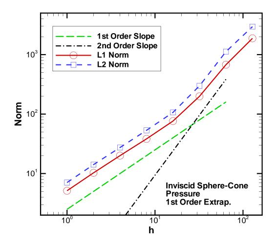
Fig. 5 Spatial error norms in pressure using one fourth of the points from the body to the outer boundary (excluding the shock).
