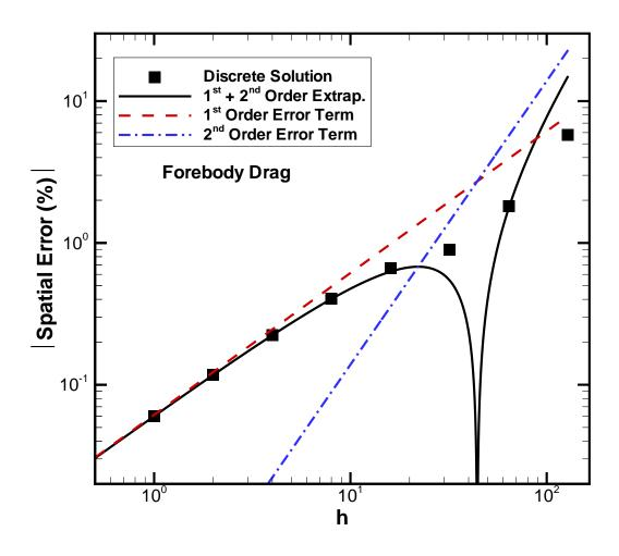
Fig. 11 Error in the forebody drag (excluding base drag) as the mesh is refined.
