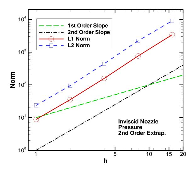
Fig. 2 Spatial error norms of pressure for the inviscid nozzle case.
