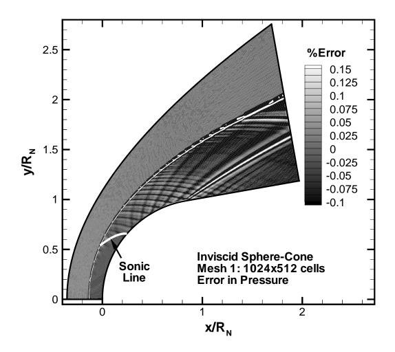
Fig. 15 Error estimates in pressure for the inviscid sphere-cone using Mesh 1 (1024×512 cells).
