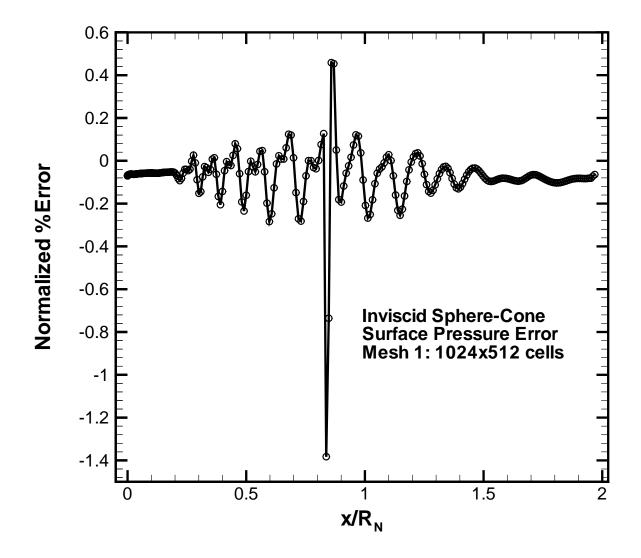
Fig. 14 Error estimates in the surface pressure for the inviscid sphere cone using Mesh 1 (1024×512 cells).
