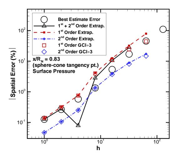
Fig. 12 Comparison of error estimates for the surface pressure at the sphere-cone tangency point ( $x/R_N = 0.83$ ).
