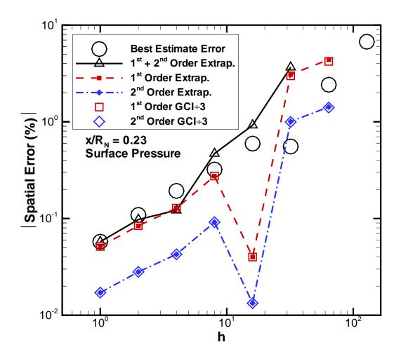
Fig. 13 Comparison of error estimates for the surface pressure ( $x/R_N = 0.23$ ).
