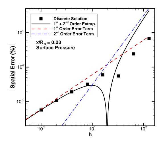
Fig. 9 Error in the surface pressure as the mesh is refined ( $x/R_N = 0.23$ ).
