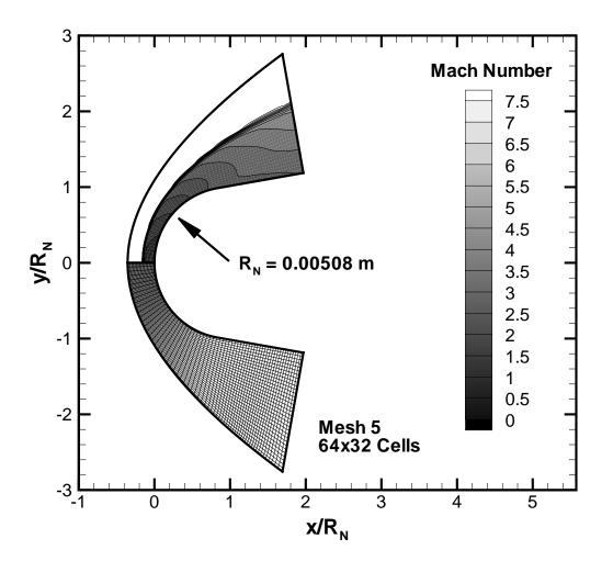
Fig. 3 Grid and Mach contours for inviscid sphere-cone.
