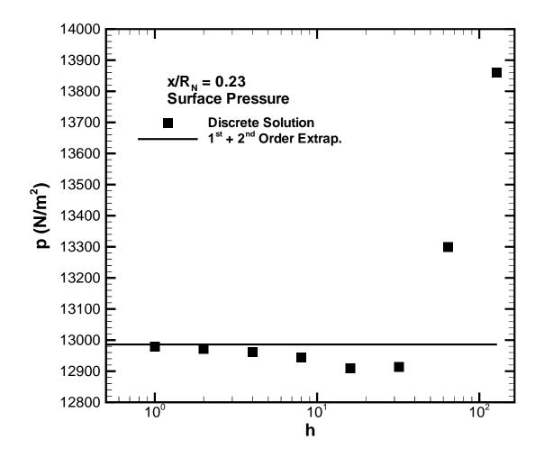
Fig. 8 Behavior of the surface pressure as the mesh is refined ( $x/R_N = 0.23$ ).
