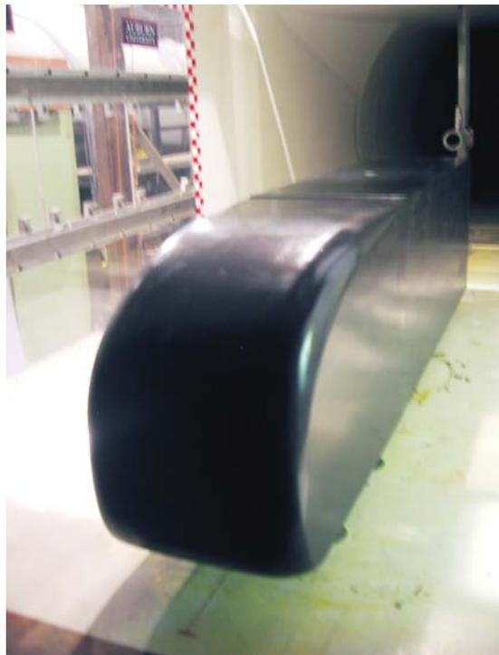
**Figure 1: Flow visualization/force model mounted in the wind tunnel test section**
