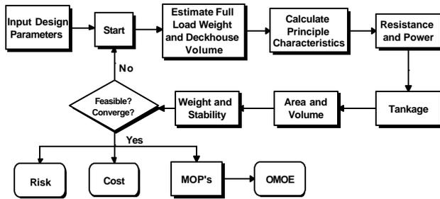
**Figure 6. Ship Synthesis Model**
