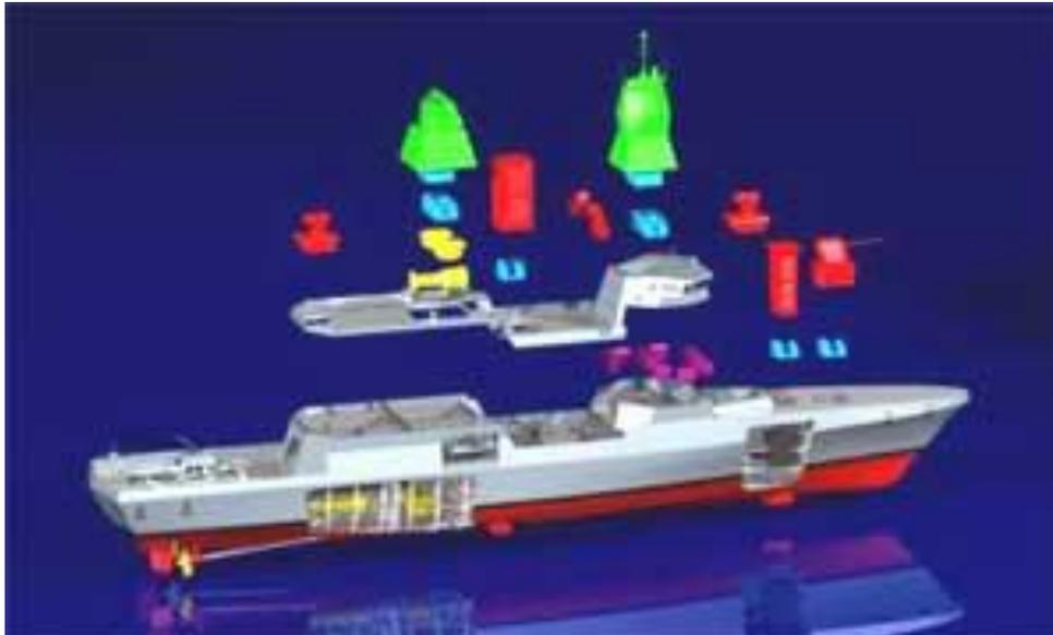
**Figure 35 Modularity Platform**
