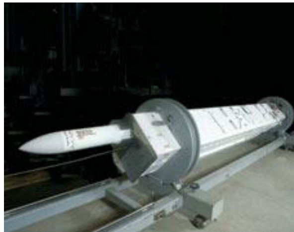
Figure 21 Quad-packed ESSM MK57 cell
