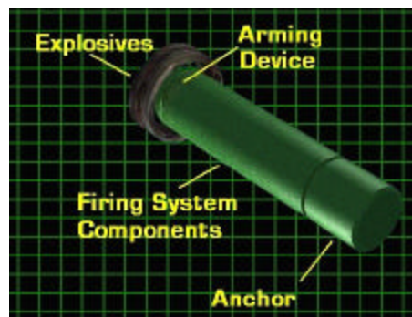
Figure 31 - Primary Components of a Bottom Mine
