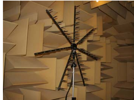
Figure 18: Photograph of the 63-element microphone phased-array.
