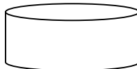
Figure 1. Cylinder. This cylinder represents an oblate axisymmetric rigid body, such as might be used to model a spin-stabilized satellite.
