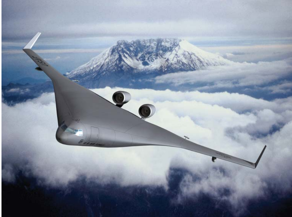
Figure 10: A Boeing BWB tanker with pylon-mounted engines (picture from Boeing).
